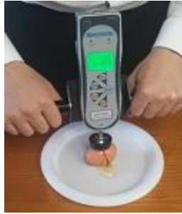
Figure 3: Force being applied to the egg laying horizontally
