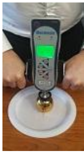
Figure 2: Force gauge with cradle being applied to bauble
