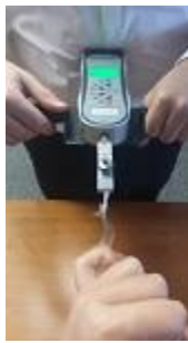
Figure 6: The wishbone being pulled apart
