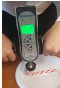
Figure 4: The force gauge on the candy cane
