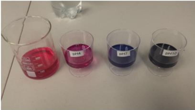
Lemonade appeared to give a deeper red colour than the pH 4 and was estimated to have a pH of 4>
