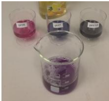
Dishwashing detergent gave a slightly purple colour so it was estimated to have a pH of around 7
