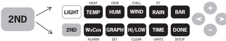
After pressing 2ND, the **2nd** icon displays on the screen for eight seconds. Key secondary functions are enabled during this time. The keys return to normal operation after the icon disappears.
