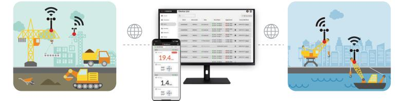
Web Portal allows users to monitor wind data and inspect the hardware storage capacity, sensor battery power, and connection status of multiple WindPro devices. Ensure the entire deployment is performing as intended and simplify maintenance efforts across sites.
