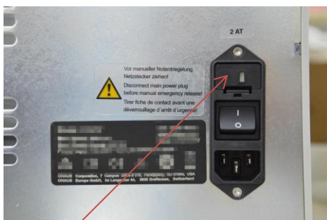
Fuse drawer with fuse 4 AT
