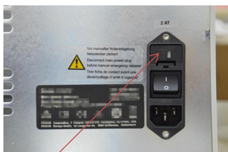
Fuse drawer with fuse 4 AT
