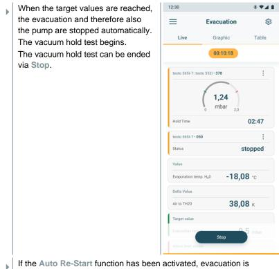
If the Auto Re-Start function has been activated, evacuation is restarted in order to restart the vacuum hold test once the target value has been reached.
