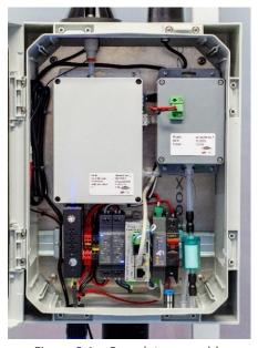
Figure 6-1 – Complete assembly DXII (setup may vary)
