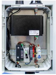
Figure 6-2 – Complete assembly DXIV (setup may vary)
