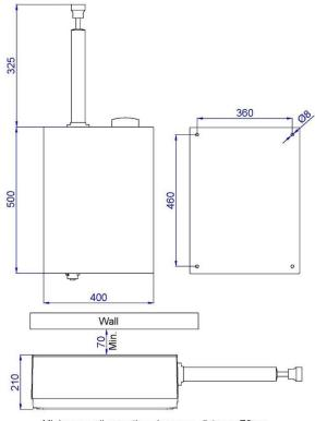
Minimum wall mounting clearance distance 70mm
