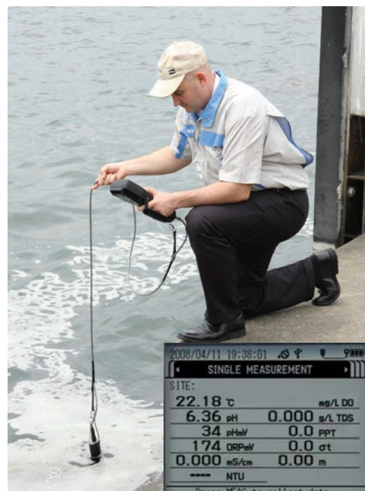
Water quality monitor displays 11 parameters simultaneously
