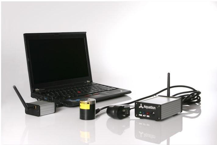
Aquation's **Classic Fluorometers** measure variable chlorophyll fluorescence including  $F_0$ ,  $F_0'$ ,  $F_m$ ,  $F_m'$ ,  $F_v/F_m$  and  $\phi_{II}$ . They can be used on the bench and in the field. The water-resistant sensor enables convenient measurement of wet material including aquatic plants and coral. USB and wireless options are available.
