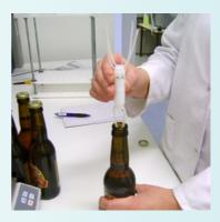
Spider cap is used inside the bottle to keep the logger centered
