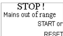
Supply voltage is monitored between 90 to 265VAC. This monitoring feature is principally used for RCD testing. Tester will not function properly below 90VAC.
