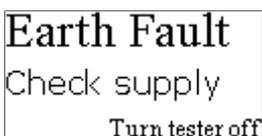
This earth fault refers to the earth supply connection to the tester. The power cord, tester or the power supply socket is damaged. The tester will not proceed to operate. This feature can be disabled.
