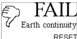
The measured value of earth resistance is above the standard earth resistance allowable.
