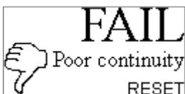
The electrical continuity of an appliance between active and neutral has not been established. Safety testing cannot proceed until establishing the cause. Ensure the appliance on/off switch is in the **on** position. Some appliances do have high impedance inputs like switch mode power supplies. Go to utilities menu to disable the electrical continuity measurement for high Z appliances.
