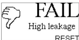
The measured value of insulation resistance below the standard leakage allowable.
