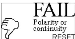
As above but applies to leads testing. Measures loss of active or neutral, active –neutral swap or possible short between active and neutral.
