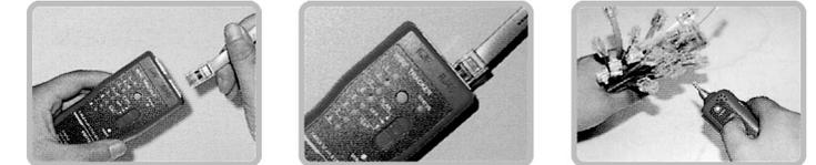
1. Directly insert network wire with RJ45 plug into the RJ45 socket of the wire tracker's emitter;
