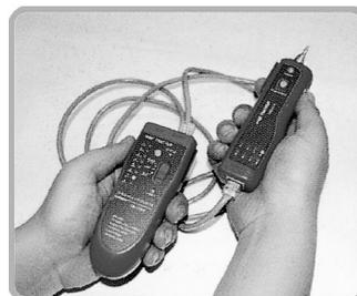
1. Insert RJ45 plug at two ends of the network wire into the corresponding sockets at emitter and receiver.
