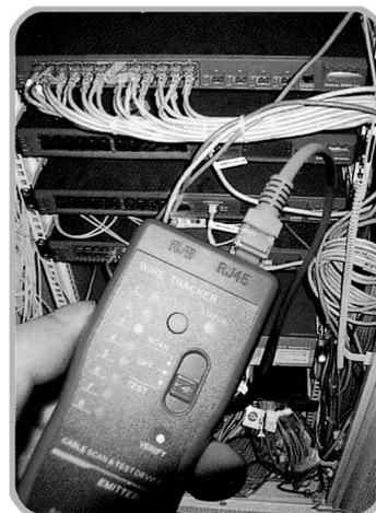
Automatic scan mode, rapidly testing, It can test correspondingly double-twisted cables 1,2,3,4,5,6,7,8 and G,meanwile,can judge wrong connection,short circuit and opencircuit.
