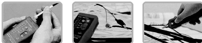
1. Directly insert telephone wire with crocodile clamp and RJ11 plug into the RJ11 socket of the wire tracker's emitter;
