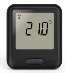
The EL-WiFi-T in the FilesThruTheAir™ range of sensors measures the temperature of the environment in which it is situated. This sensor is typically accurate to ±0.5°C/ ±0.1°F (-10 to +50°C/ -14 to +122°F). Data is streamed wirelessly over any WiFi network and can be viewed on a PC using free software or on the FilesThruTheAir™ Cloud.
