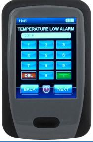
6. Enter precise alarm values with the numbered touchpad.
