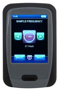
4. Set the scale (in this case °C or °F) and the sample frequency.
