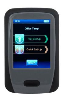
2. Your options are "Full Set-Up" or "Quick Set-Up." Choose "Quick-Set-Up" if you've already configured your EL-USB data logger and simply wish to begin recording a new file. Choose "Full Set-Up" to configure your data logger.
