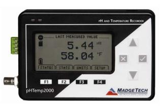
readings per channel. The pHTemp2000 will directly connect to many commonly used pH, ORP and ISE electrodes through a female BNC connector mounted on its side. Temperature is measured by directly connecting an RTD to the pHTemp2000. Temperature compensation is automatically done internally to the unit.
